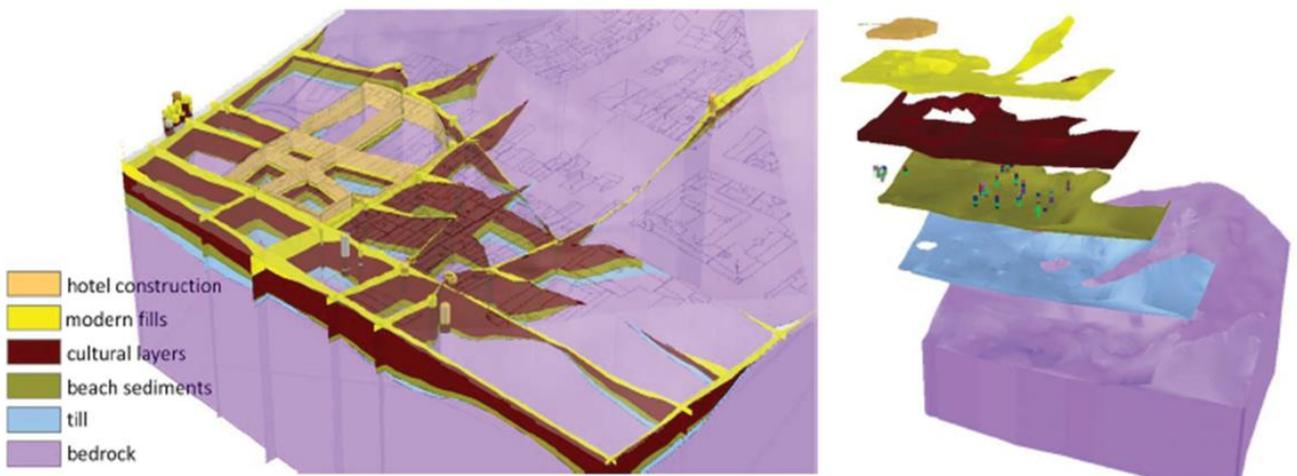
Modell of layers in the subsurface below Bryggen. The cultural layers, consisting mostly of organic material from human waste, can be more than 10 meter thick. Underneath are natural sediments beposited by the fjord and glacier, on top of bedrock. The walls of the modern hotel, sheet pile wall, is marked with orange in the modell (Source: De Beer, 2015).
