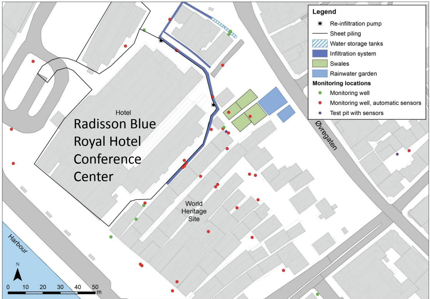
Overview map of mitigation measures carried out by the Groundwater Project, including locations of monitoring wells for measurement of groundwater level, temperature and sampling. Map: Anna Seither, Geological Survey of Norway.
