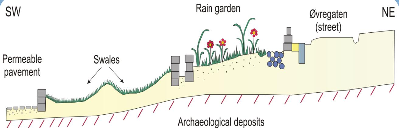
Section of the sustainable water management "treatment train", with rainwater garden, swales and permeable pavement. Drawing: Johannes de Beer, Geological Survey of Norway.
