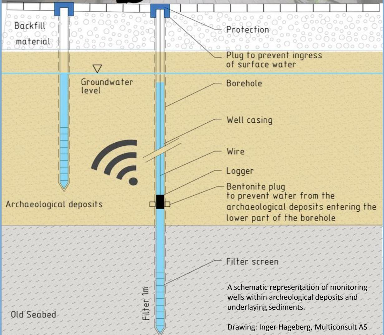
A schematic representation of monitoring wells within archeological deposits and underlying sediments.
